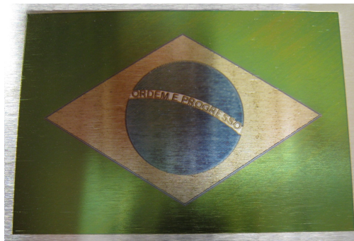
Color Marking on Stainless Steel
