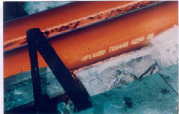
HOT SPRAY I-DENT® MARKING ON 1800°F HOT STEEL
